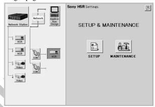
Use the (SETUP) icon to make HSR-1/1P/2/2P settings from the Web page. Clicking the "Setup" icon displays the "SETUP MENU".
